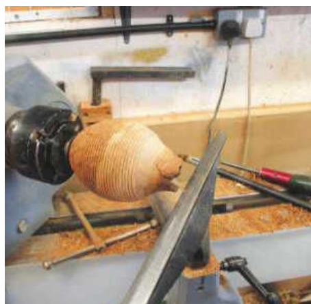
STEP 18. I feared this might happen: as I wanted to turn the piece thin, the depth of the bark was likely to cause a problem. A split has appeared and will need to be repaired if I want to keep the top intact
